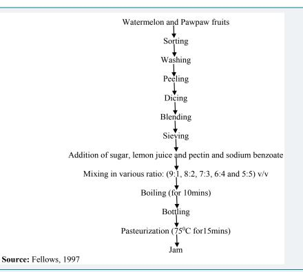
Figure 1: Flowchart for the production of watermelon-pawpaw jam.
